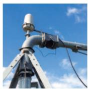
The flexible connection between the center tower and the spray of pivot absorb the stress caused by hilly condition, effectively guarantee the longer operating life of the
