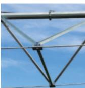
The arched triangle of the span ensure the stable operation under hilly condition or big land slope.
